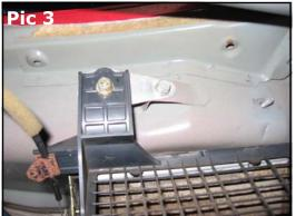
NOTE: The bracket for the upper blower mount is not necessary if you installed the Optional Dash Bar. The upper blower mount will wedge between the dash bar and the body as shown in Pic 4.
